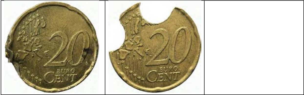
c. Bent and punched (due to impacts)
